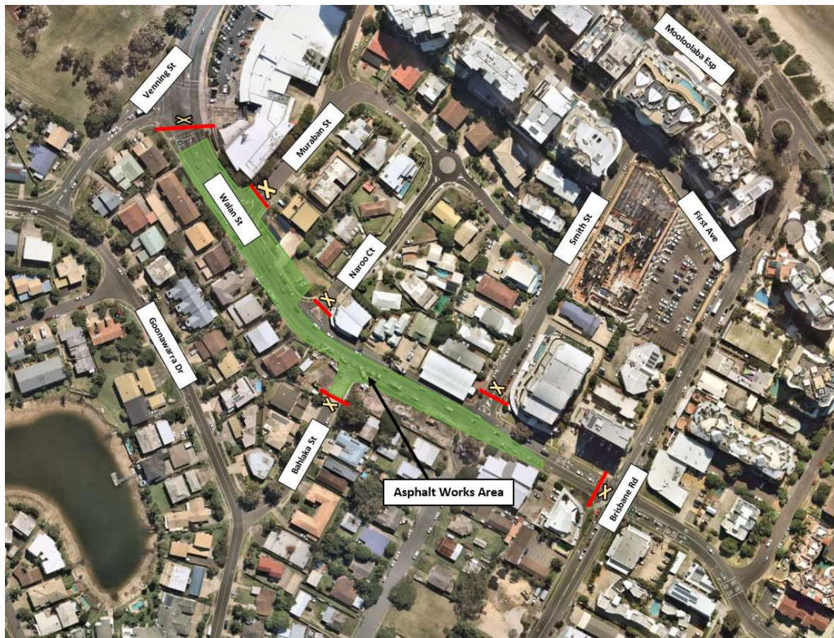
FIGURE 1: Road resealing section and temporary changes to traffic conditions Monday 23 November to Thursday 26 November 6am – 6am/24 hrs (day and night works)
